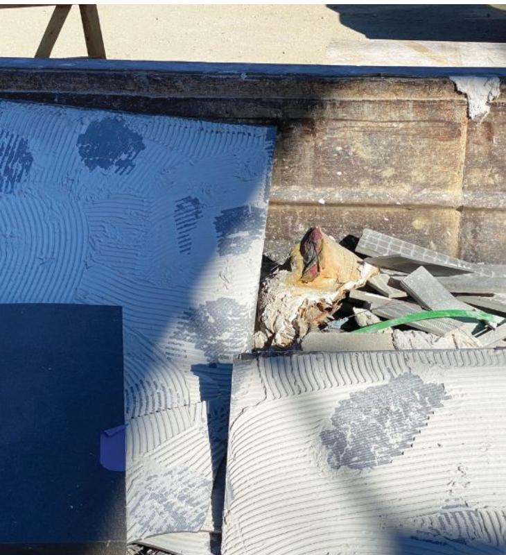
The original installers tried spot bonding these large-format tiles, placing dollops of extra thinset on the back in the hopes of promoting better adhesion. The high points on the thinset layer indicate where they placed the dollops. The spots with missing material show where the tiles came loose from the dollops.
