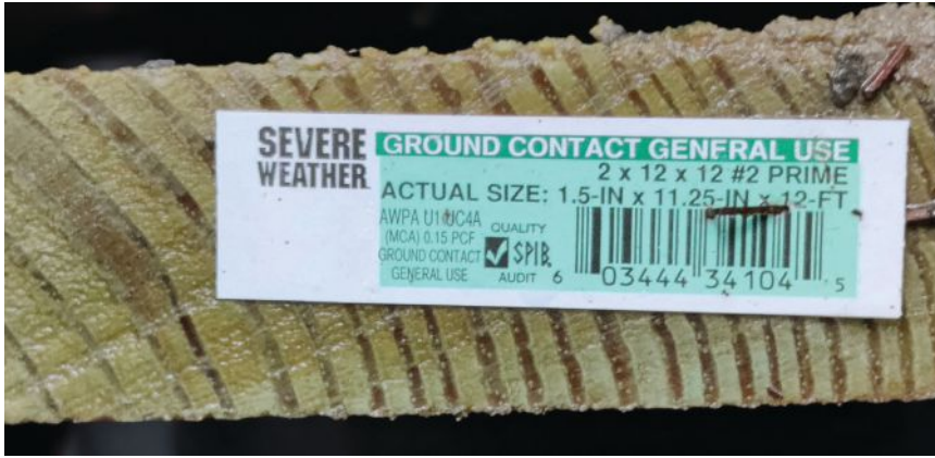
Preservative treatment lumber tag on one end gives the size of the 2x12, along with the AWPA UC4A level that indicates it is suitable for “Ground Contact.”
