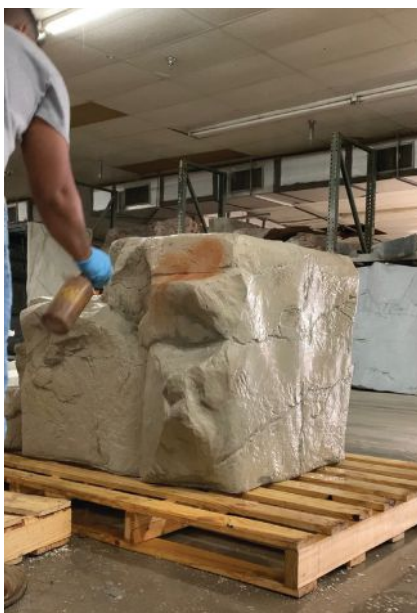
It takes several layers of color to create the shading and variegation found in natural stone.
