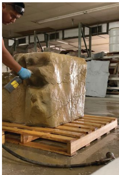
It takes several layers of color to create the shading and variegation found in natural stone.
